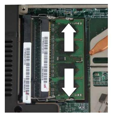
7 If you are removing a module, gently press outward on the clip at each end of the memory module until the module tilts upward.
